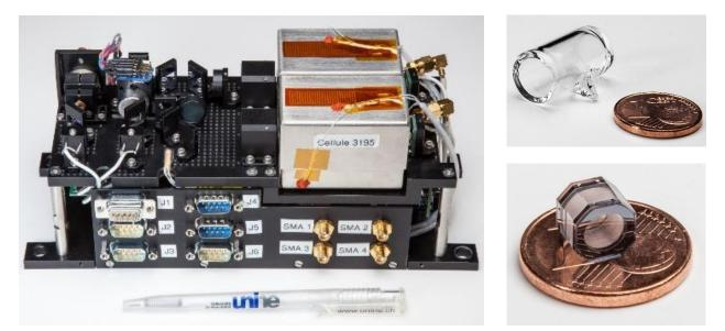
Left: prototype of laser-pumped Rubidium atomic clock for next generation satellite navigation system (Galileo). Upper right: glass-blown Rubidium vapor cell for laser wavelength stabilisation (for atomic clocks and Lidars). Lower right: micro-fabricated Rubidium vapour cell for next generation chip-scale atomic clocks.
